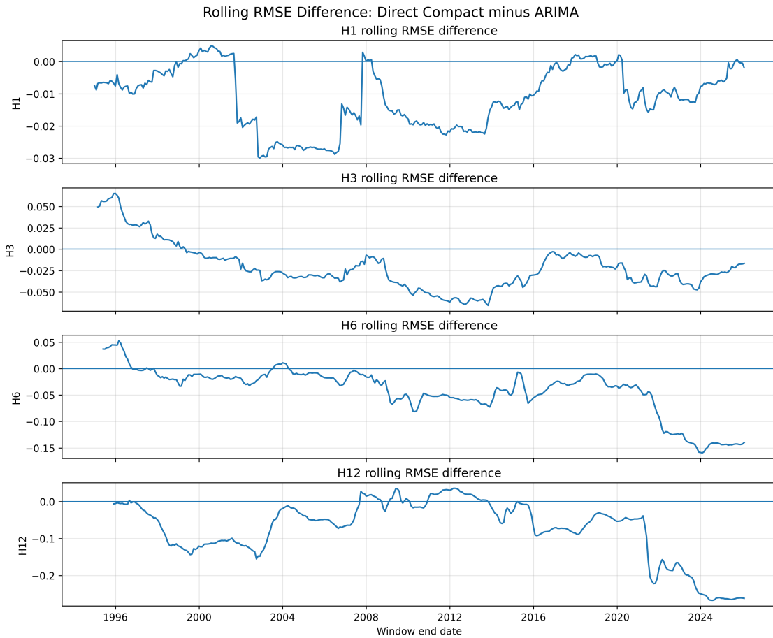
Figure 4: Rolling RMSE Difference: Direct Compact minus ARIMA Negative values indicate rolling windows in which the direct compact model outperforms the ARIMA benchmark.
